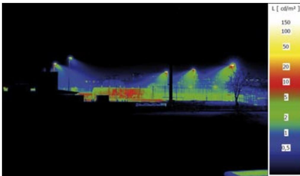
Fig. 41: Example of optimized lighting at a sports ground (luminance measurement using inverse colour image)
