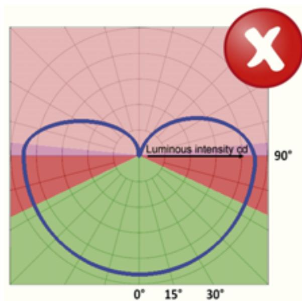
Fig. 35: Intensity distribution curve of an old-style street light lamp suspended on cables in the middle of the street
