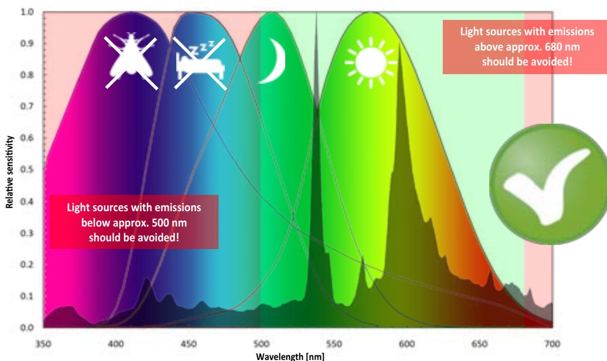
Fig. 22: Spectrum of a metal halide lamp
