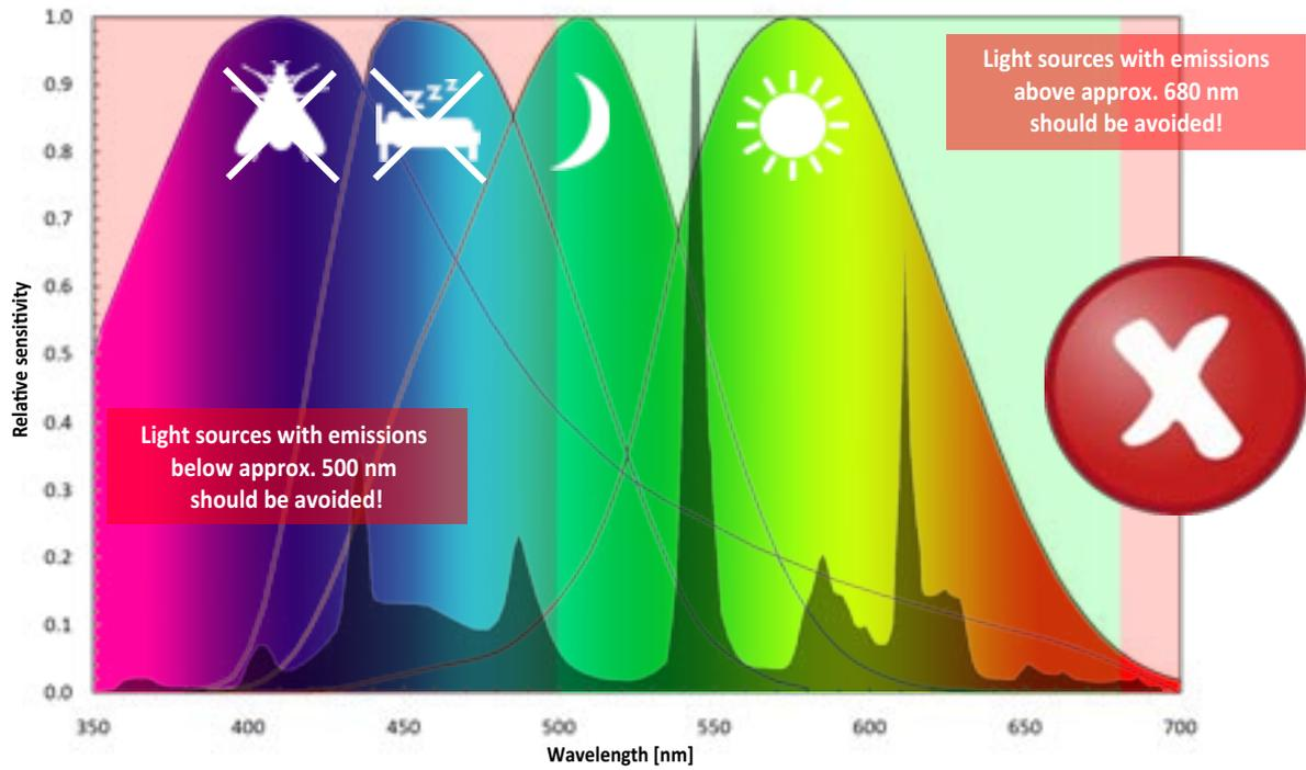
Fig. 20: Typical **spectrum** of a fluorescent lamp with a correlated color temperature of 5000 K
