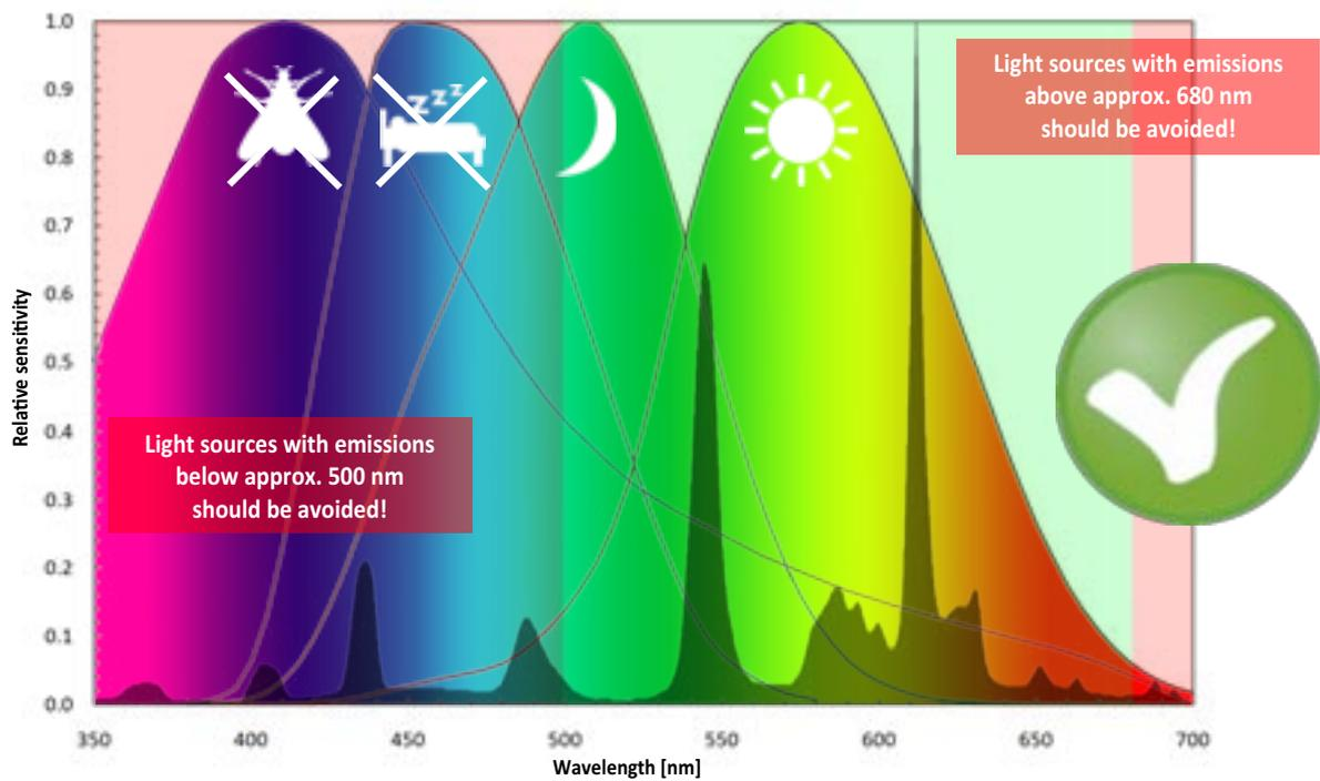
Fig. 21: Spectrum of a fluorescent lamp or energy-saving lamp with a correlated color temperature of 3000 K and a low blue component
