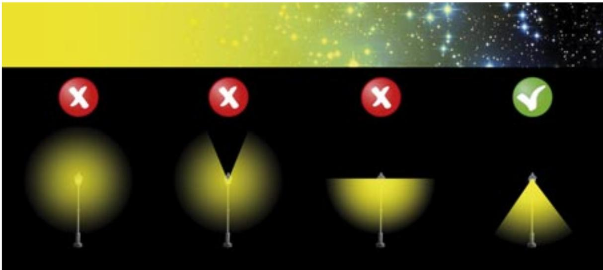
Fig. 30: Illustration showing the ideal beam geometry
