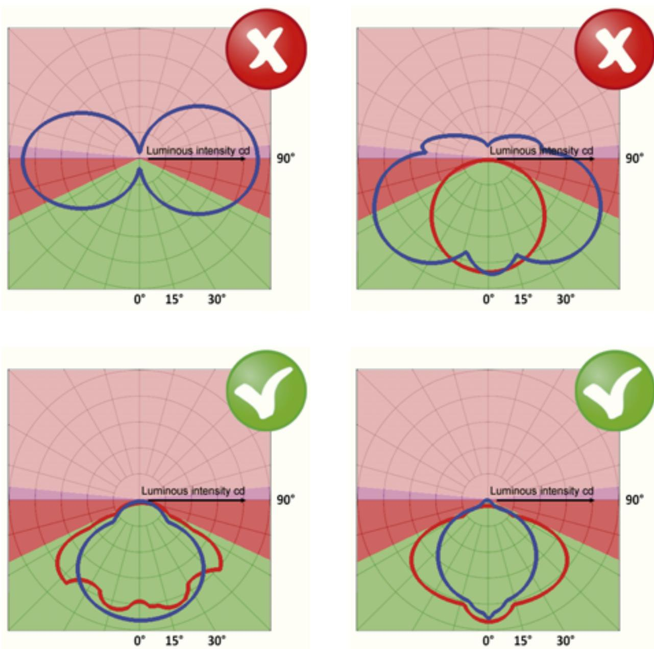
Fig. 36: typical luminous intensity distribution curves
