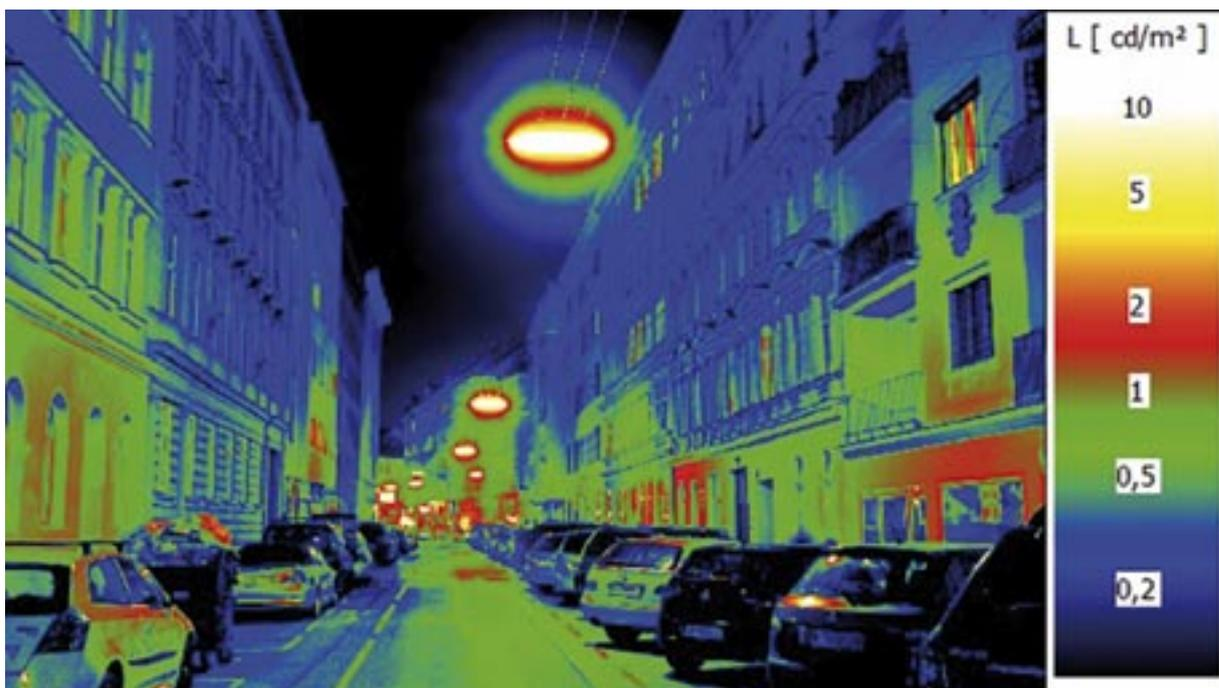
Fig. 32: Previous lighting of a street in Vienna using fluorescent lamps
