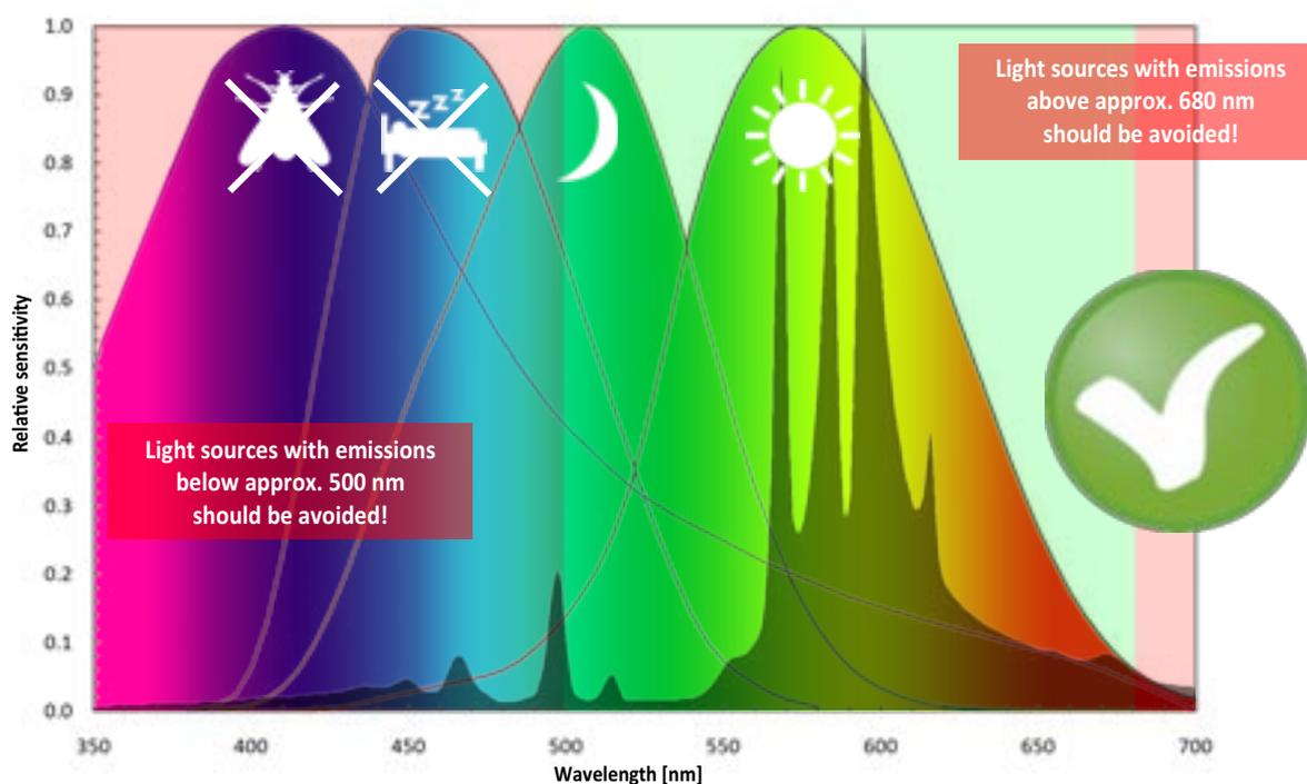
Fig. 26: Spectrum of a high-pressure sodium vapour lamp
