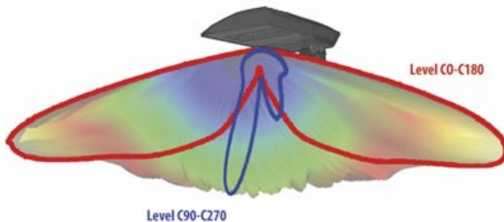
Fig. 34: Illustration of two measuring levels of a luminous intensity distribution curve for a street lamp
