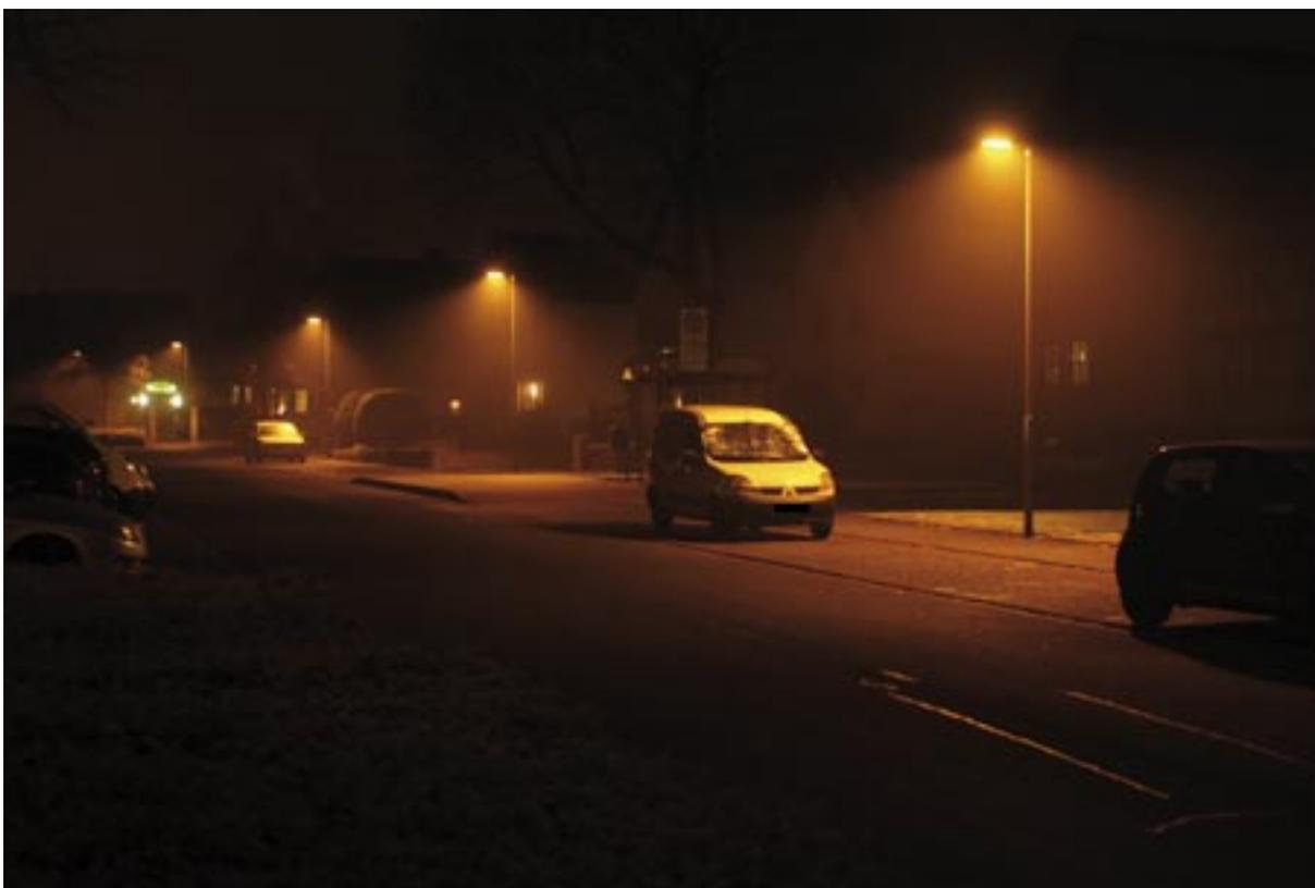
*Fig. 29: Shielded lamps only illuminate the road and do not create glare*
