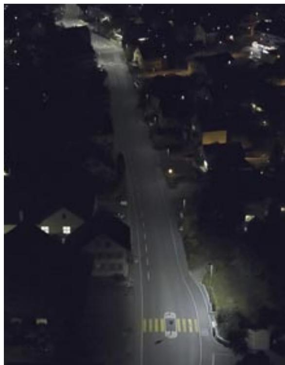
Fig. 39: Traffic-sensing light in Urdorf (CH): Illuminance varies between 100 % (left) and 40 % (right) depending on the volume of traffic
