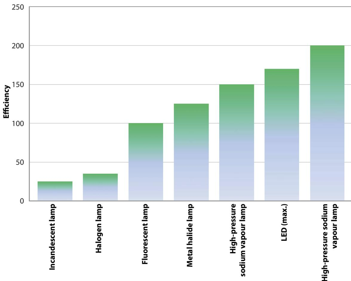
Fig. 28: Efficiency comparison of light sources (efficiency = luminous efficacy)
