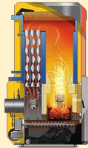
Wood chip boiler
