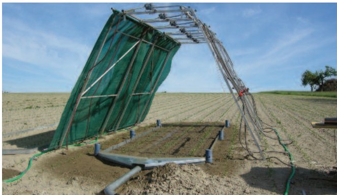
Abb. 20: Regensimulator BAW Petzenkirchen (Variante CT)
