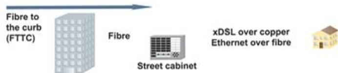
Abbildung 62: Fiber-To-The-Curb (FTTC) [15]
